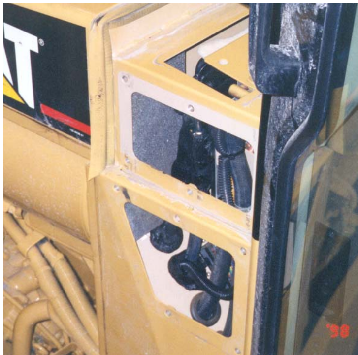
Evaporator assembly showing hoses.
