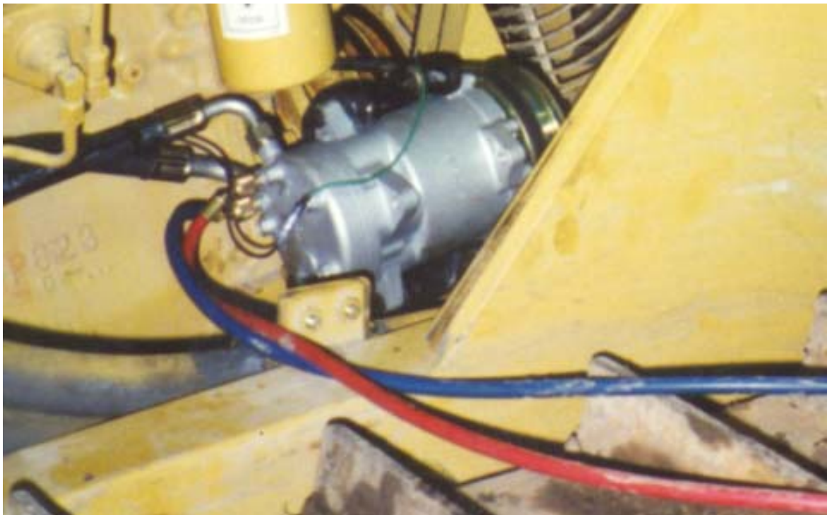
Compressor mount and compressor in place. (Old style compressor)
