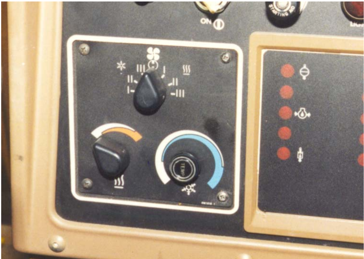
Thermostat in location on dash control panel.
